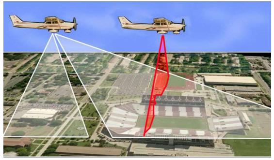
Pictometry has developed a proprietary method of utilizing the combined nadir imagery, LiDAR raw data and ground control to greatly increase the efficiency of the mosaic process.
